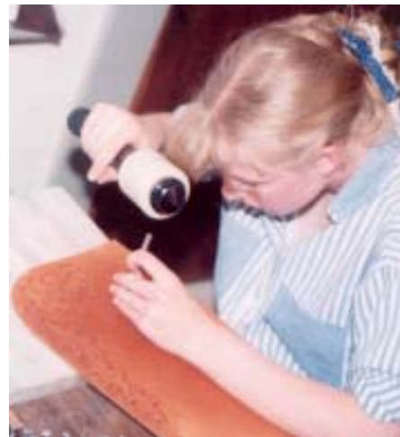
Lacy Rose stamps oak leaf patterns into leather. Rose, who is a talented artist, drew the leaf patterns as well as running horses for the saddle she crafted.
