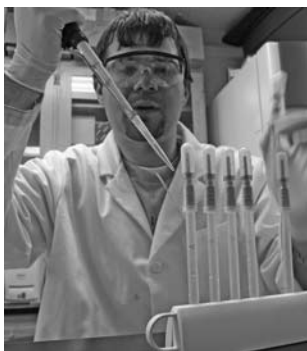
John Willford introduces bacteriophages to the Phast Swab. The tubes are incubated for an hour and a half then the tops snapped, which releases a substrate into the bottom of the tube to react with an enzyme.
